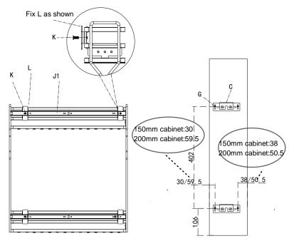
Assemble J1 into J2 and pull & open the basket for times to insure the slide in the right position.
